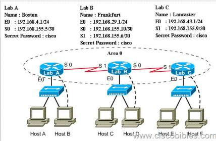
The question mentioned Boston router was not configured correctly or incomplete so we should check this router first. Click on PC-B to access the command line interface (CLI) of Boston router. Boston>enable (type **cisco** as its password here) Boston#show
