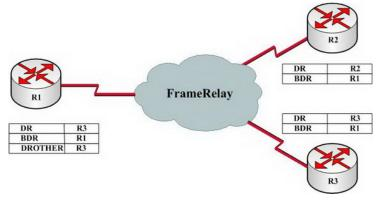
The reason that this problem occur is the network topology of Frame-Relay is not full meshed. When R3 is establishing neighbors with R1, R3 know not the existence of R2. And when R2 is establishing neighbor with R1, R2 know not R3. At this time, the network is running two different OSPF auto systems.
